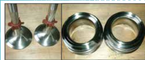
M/E EXHAUST VALVE SPINDLE AND SEAT AFTER RECONDITION.
