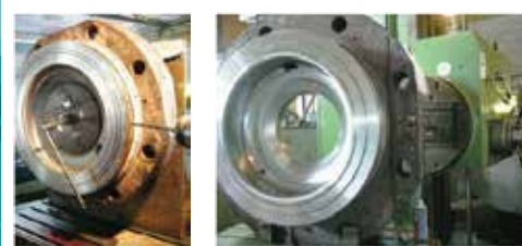
VARIOUS TYPE OF M/E CYLINDER COVER AFTER REPAIR AND BORING IN PROGRESS.
