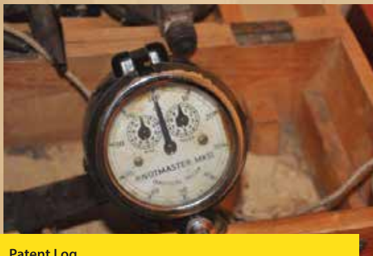
Patent Log (The Patent Log came with the advent of steam ships)
