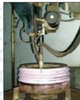
M/E PISTON CROWN AUTO SUB ARC WELDING IN PROGRESS
