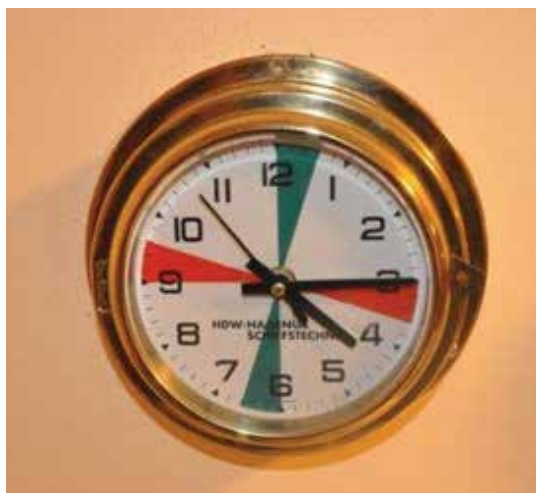
Ship's Clock with Silence Period. All stations using 2182 kHz were required to maintain a strictly enforced three-minute silence and listening period twice each hour, starting at h+00, h+30.
