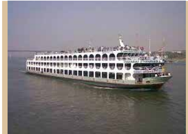
Figure 2 A Triple-decker passenger vessel resulting a large windage area with a shallow draft
